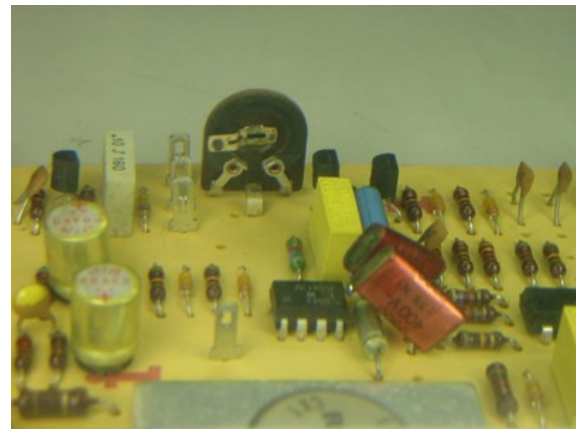
The modified capstan controller board.
